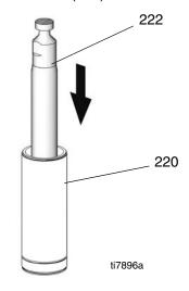
5. Grease top inch or two of piston rod (222) that will go through the cylinder throat packings.
